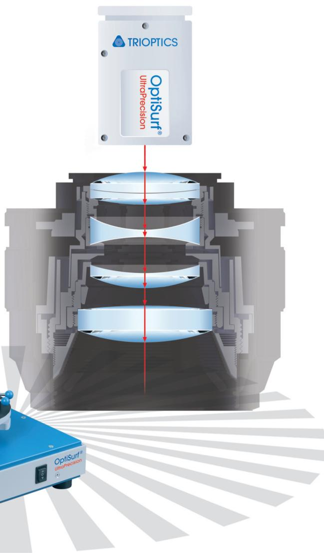
OptiSurf® is the ideal tool for non-contact center thickness and air gap measurements of single lenses, flat optics and within optical systems. The instrument is based on low coherent interferometry and measures all surface distances in an optical system with an accuracy up to 0.15 µm in one scan.
