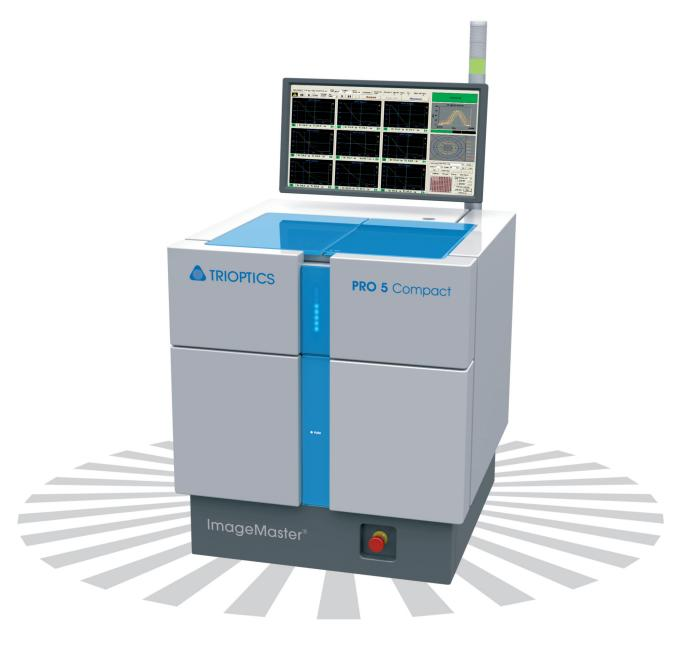
The new ImageMaster® PRO 5 Compact is the entry level production MTF test station for qualifying mobile phone lenses and other miniature lenses with an effective focal length between 1 and 12 mm. It features an accuracy of 2 % MTF on-axis and a production speed of up to 1500 UPH. Ergonomically designed as a space saving table top instrument it is optimized for clean room production.
