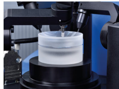
OptiCentric® Cementing cements two hemispherical lenses of different diameters
