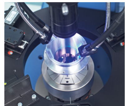
OptiCentric® Bonding with three actuators for alignment of the lens in the cell
