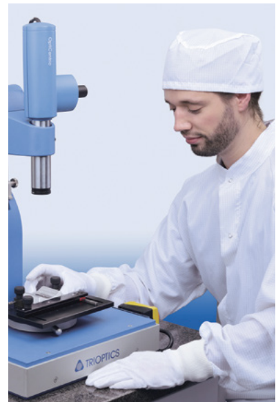
An operator measures a cylinder lens
