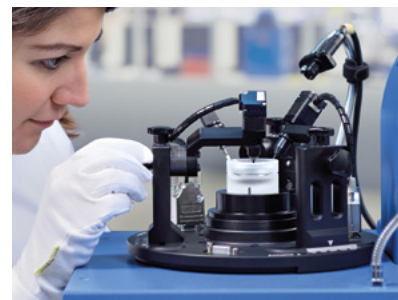
Employee performing automated lens alignment and cementing
